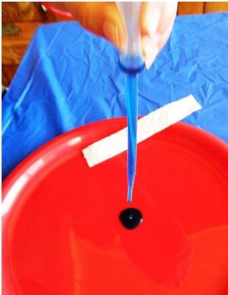
**Step 1:** Fill the dropper with blue-dyed water and place a small pool of that water on the plate.
