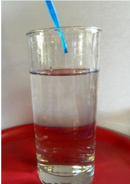
**Step 1:** Fill a dropper with blue-dyed water and add a drop to the clear glass of water.
