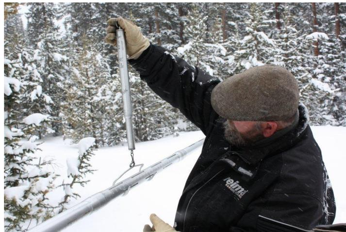
Snow sampler is being weighed to determine the water content of the snow
