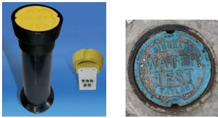
**General:** The Water CP Test Station offers the versatility of being buried in or near street pavement. Each 5.25-inch lid shall be painted "Blue" and shall have "Water Test" cast into the Heavy Duty H20 rated lid. The body shall be 15 inches in height and made of high impact plastic. A 5-terminal test board shall be attached to the lid. This test box will be used in conjunction with Cathodic Protection Test points and systems.
