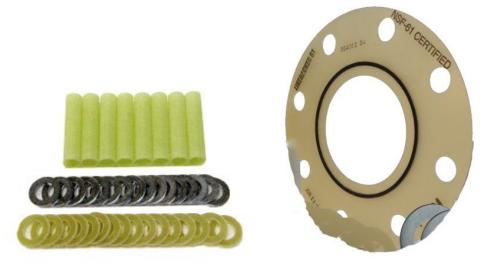
**General:** Flange insulation Sleeves and Flanges are used as a means in controlling losses due to corrosion. They can be used to increase the effectiveness of cathodic protection systems and confine or eliminate electrolytic corrosion. Flange Insulation Kits should be obtained in ANSI Class 150 or 300 depending on the Flange Configuration needed and shall include Insulating Sleeves and GRE/ZPS Washer sets. Isolation Flange Gaskets are also used to aid in corrosion losses.
