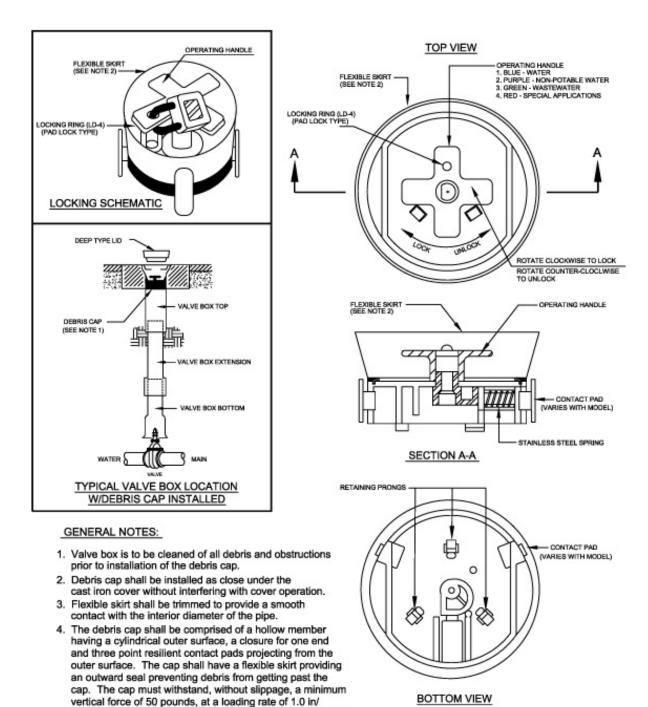
minute. The cap shall be molded using General Electric ABS #him 4500. The cap shall have retaining prongs to retain
