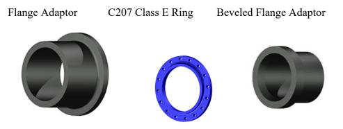
Flange adapters shall be made with sufficient through-bore length to be clamped in a butt fusion-joining machine without the use of a stub-end holder. The sealing surface of the flange adapter shall be machined with a series of small v-shaped grooves (serration) to promote gasket-less sealing, or restrain the gasket against blowout. A Beveled Flange Adaptor is for use with Butterfly Valves.
