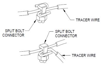
Once the wire split bolt connector is in place it shall be encapsulated with a Split Bolt Housing or Tape Wrapping.
