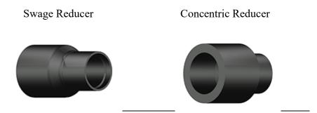
Swage reducers are preferred for use when reducing one nominal pipe size. When reducing more than one size, the Contractor needs to be aware that the reducer length can be longer than expected due to step down from each size. Check with the manufacturer for reducer lengths.
