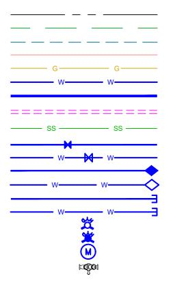
DEVELOPER PHASE LINE EASEMENT LINE EXISTING ROW/PROPERTY LINE EXISTING CURB LINE EXISTING GAS MAIN EXISTING WATER PROPOSED WATER EXISTING NON POTABLE WATER EXISTING SEWER VALVE (PROPOSED) VALVE (EXISTING) BLOWOFF (PROPOSED) BLOWOFF (EXISTING) PLUG (PROPOSED) PLUG (EXISTING) EXISTING FIRE HYDRANT PROPOSED FIRE HYDRANT EXISTING/PROPOSED METER PIT BACKFLOW PREVENTION ASSEMBLY (BFP)
