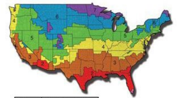
Department of Energy Recommendations for Attic Insulation
