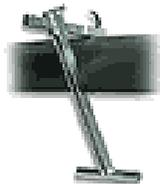
Internal fusion beads between HDPE fittings and Pipe Pup additions shall be removed and all additional internal beads created during manufacturing (if required) after the allowable cooling time for bead removal using a suitable bead removing tool specified for HDPE pipe. The bead removal tool shall not induce any slits, gouges or defects in the pipe wall, as recommended by the manufacturer. External beads must be removed to provide access for rings to be applied to fittings, where applicable.
