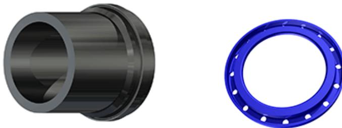
MJ Adapter 4” through 24” must be provided with a Stainless Steel Stiffener (included in the manufactured fitting). All MJ Adapters shall be provided with a Heavy Duty Back-up Ring and Kit (*AWWA C110* with minimum 8 mils fusion bonded epoxy coated follower/back-up ring). The kit needed shall also include bolts and nuts, Grade 3 or higher and long enough to accommodate the added length of HDPE fittings to attach to valves or other appurtenances.
