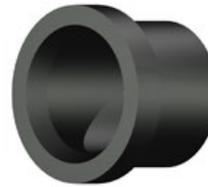
Flange adaptors shall be made with sufficient through-bore length to be clamped in a butt fusion-joining machine without the use of a stub-end holder. The sealing surface of the flange adaptor shall be machined with a series of small v-shaped grooves (serration) to promote gasket-less sealing, or restrain the gasket against blowout. A Beveled Flange Adaptor is for use with Butterfly Valves.
