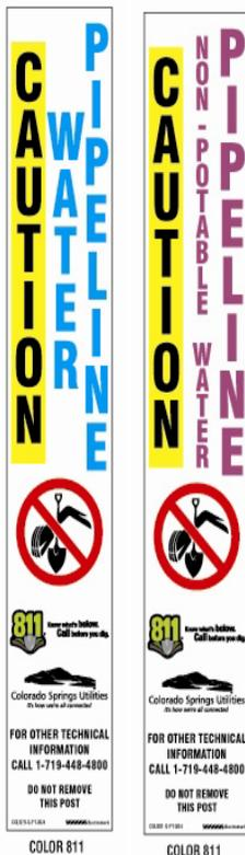
**General:** Line markers are to be installed with Colorado Springs Utilities decal and telephone number.
