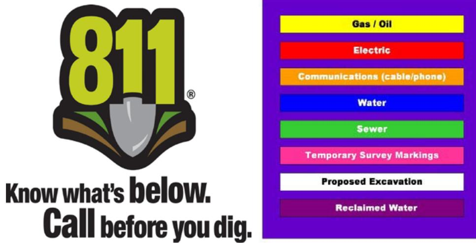
**Figure 5-1: Uniform Color Code for Underground Utilities**
