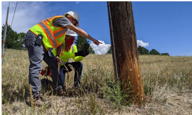
Wood pole inspectors investigating a pole as part of our Wood Pole Testing and Treatment program.
