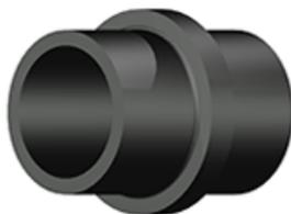
Wall anchors shall be manufactured according to *AWWA C906* with the PE 4710 cell classification and shall be manufactured as one piece, compatible to the HDPE pipe being placed and shall be rated for internal pressure service at least equal to the full-service pressure rating of the mating pipe. The HDPE wall anchor shall be fused to the pipe and supported to allow for the placement of a concrete reverse anchors (CRA).
