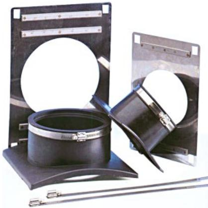
**General:** Saddle Taps may be an EPDM rubber gasket with locating/centering ring with corrosion resistant Series 300 austenitic stainless steel apron fastened with 300 series stainless steel bands, full 9/16” width band with a cadmium plated carbon steel 5/16” shouldered hex head slotted screw.
