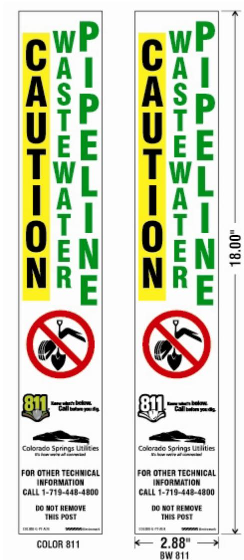
**General:** Line markers are to be installed with Colorado Springs Utilities decal and telephone number.
