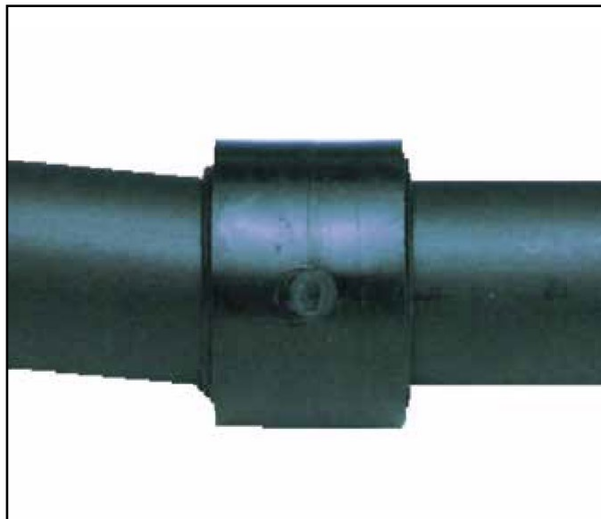
Excessive Stab Depth Caused by Failure to Use a Cold Ring to Use a Cold Ring
