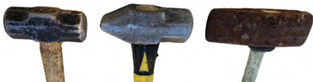
Figure 7–22. Heads of common hammers for rock work (left to right): engineer's hammer, cross peen (a.k.a. blacksmith hammer), and mason's hammer. The mason's hammer is made of soft metal designed to be hit with a sledge for rock shaping. USDA photo by Jess May.
