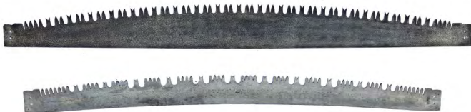
Figure 7–28. Blades of bucking (top) and felling (bottom) crosscut saws. USDA photo by Matt Able.
