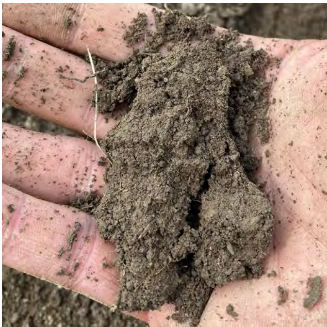
Figure 2–10. Loamy soil is a mixture of sand, silt, and clay and is great for trail building. USDA photo by Matt Able.
