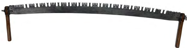
Figure 7–27. Ribbon-style felling crosscut saw with handles. USDA photo by Kerry Wood.
