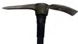
Figure 7–7. Pick mattock and cutter mattock heads. USDA photo by Matt Able.
