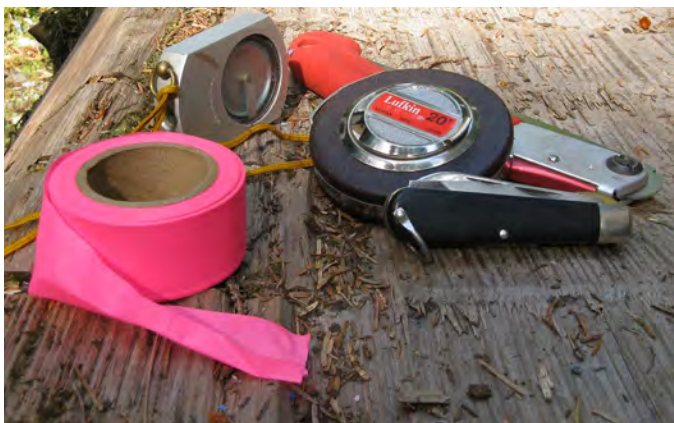
Figure 6–5. A few essential tools for scouting and laying out a trail: clinometer, flagging, diameter tape (also called forester tape), pocketknife, and folding handsaw. Tongass National Forest, Alaska. USDA photo by Laurent Deviche.
