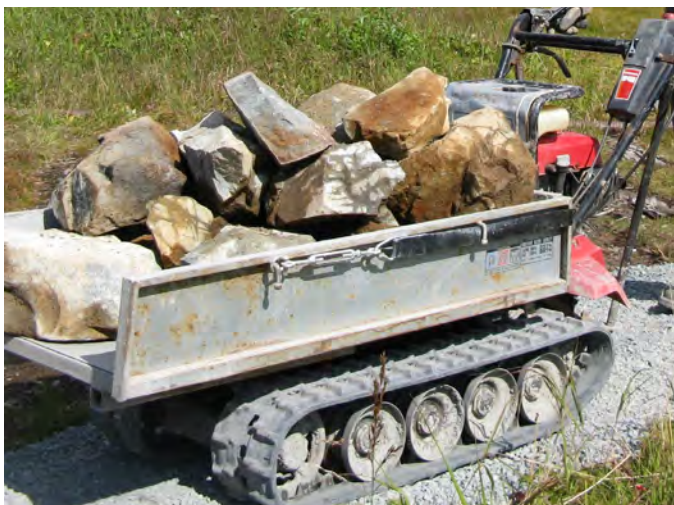
Figure 7-12. Motorized carrier being used to transport rocks. Tongass National Forest, Alaska. USDA photo by Laurent Deviche.
