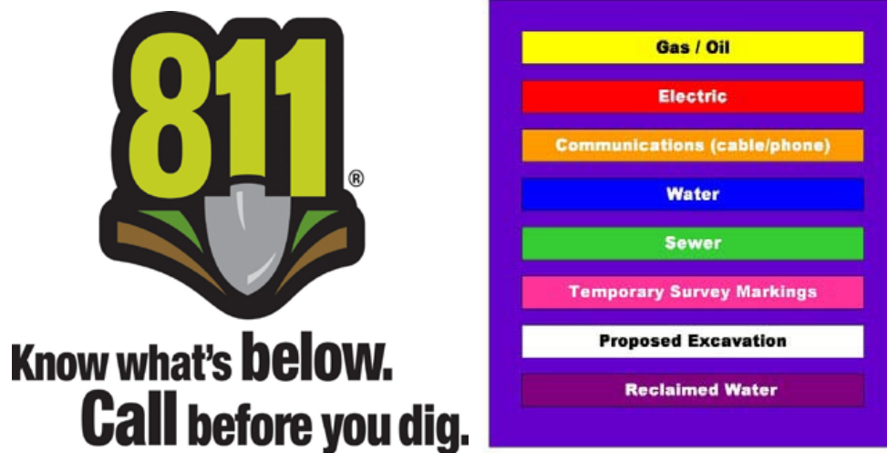
Figure 5-1: Uniform Color Code for Underground Utilities
